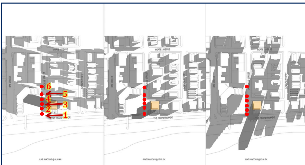
Figure 13: Drawing PN.0399/ 004 showing June shadows of the proposed development. The approximate locations of the trees are denoted by the red dots.
